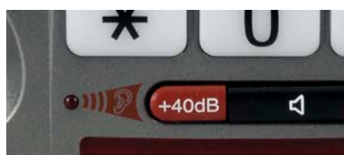
Boost Button increases receiver volume
