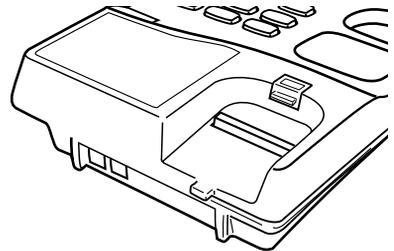
4. Insert the HANDSET RETAINER back into it's slot
