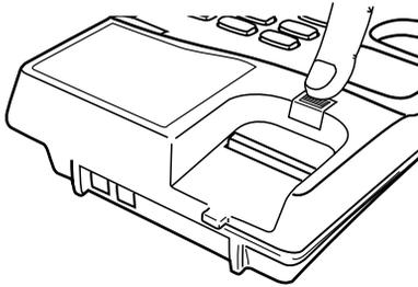
2. Push the HANDSET RETAINER out of the slot
