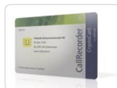
A Crypto Card is an IC card that can be placed in the card reader of the recorder. Recordings that are made using a Crypto Card are in encoded format and cannot be listened to without a Crypto Card of the same set. The Call Recorder Access System supports the use of an IC Card Reader for the PC and can play the Crypto Card encoded recordings or can convert them to generic audio formats. In this way, the Call recorders and the software can offer a high level of security without any inconvenience.
